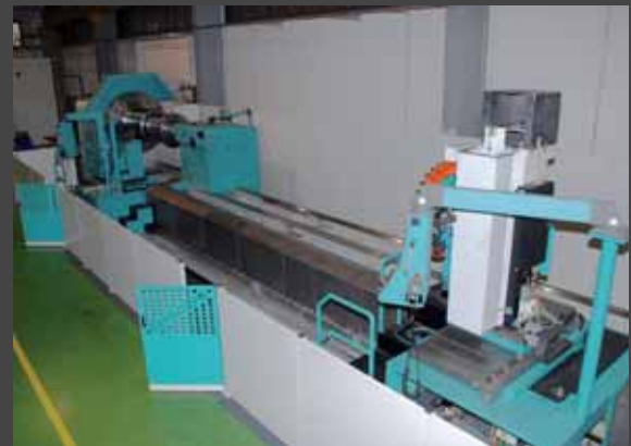
Machine equipped with two carriages, the second one with milling unit column and automatic tool-change system.
