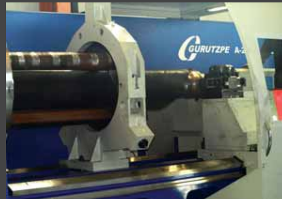
Detail of the machining process with pieces of big eccentricity.
