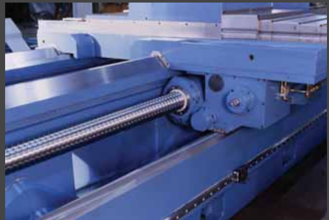
Detail of the static ball-screw with rotating nut.
