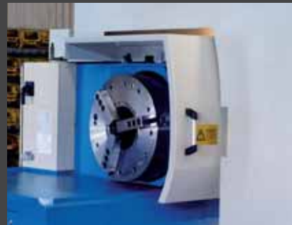
Detail of a headstock with big bore and automatic rear chuck.
