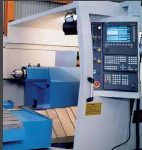
Detail of an in-built CNC in the door.
